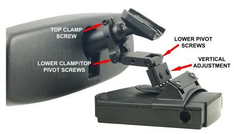
7 - Install the RD onto the mount. Make the necessary adjustments as shown above. Using the vertical adjustment, we recommend you adjust the RD as close to the bottom of the mirror as possible.
